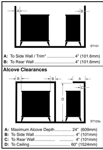
Fig. 2 Minimum wall clearances.
